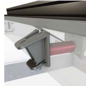
ANTI-CRUSH TUBE BETWEEN RAFTER LUGS
